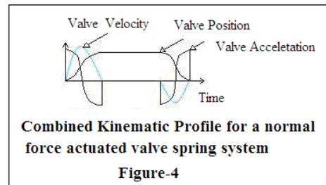
Combined Kinematic Profile for a normal force actuated valve spring system
