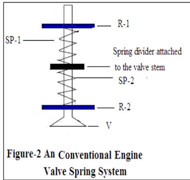
Figure-2 An Conventional Engine Valve Spring System
